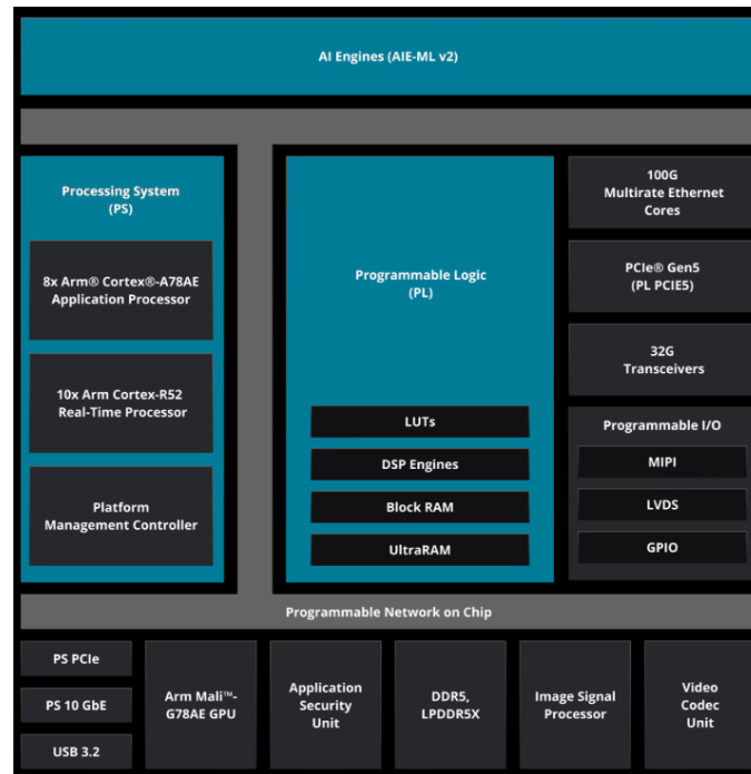
VERSAL™ Prime & AI Edge Series Gen2 Block Diagram
