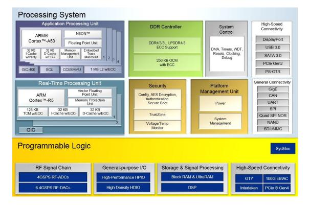
Applications processing unit (APU) with quad-core ARM® Cortex™-A53 processors up to 1.5GHz:
